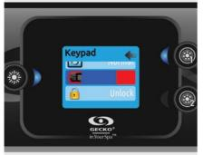
With the in.k506 equipped with a selectable rim light color modul: If the "RGB backlight" option is enabled in the spa configuration an option will appear to allow selection of the keypad rim light color.
